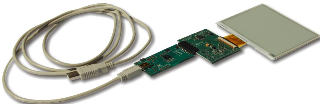
Figure 2.2: USB2TCM\_v1.1 connected to a TCM-P441
