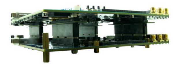
1. HMF3C Height extension adapter card Part No: S0171 Weight: 200g
