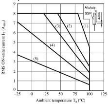
Fig.3 RMS ON-state Current vs. Case Temperature
