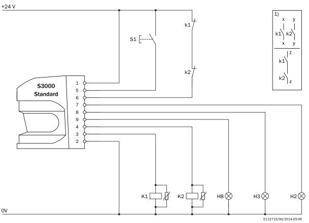
S3000 Standard in conjunction with relays/contactors
