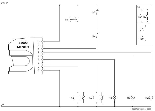
S3000 Standard in conjunction with relays/contactors
