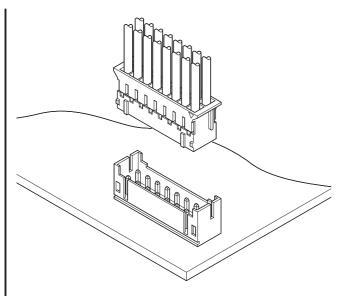
This is a 2.0mm pitch, crimp style, doublerow, wire-to-board connector. It is designed to meet the demand for highdensity and low-profile connection.
