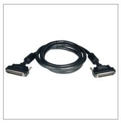
**Description**Multi-platform SCSI III external peripheral cable HD68M/M. This 10ft cable is designed to connect two SCSI III (fast and wide) or SCSI II devices together. Supports all legacy transfer rates through Ultra 320. Manufactured using double shielded 34 twisted pair high impedance cable. Constructed with low-capacitance, impedance matched, 28 AWG, stranded, tinned copper cable with insulated in polypropylene.
