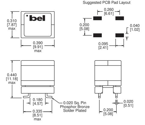
Dimensions are in inches [millimeters]. Standard dimension tolerance is ±0.005 [0.13] unless otherwise noted.
