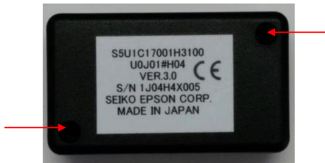
Figure 5.1 Screw Positions on the Bottom Cover
