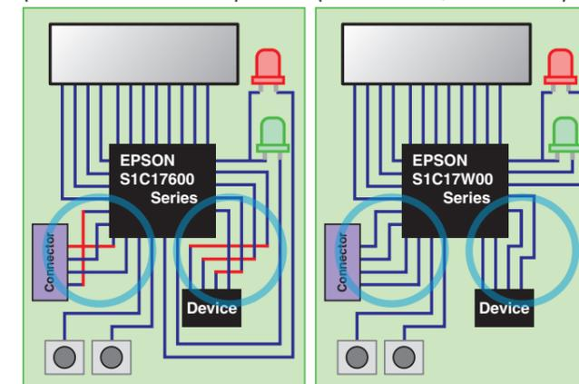
Terminals can be allocated freely using software.
