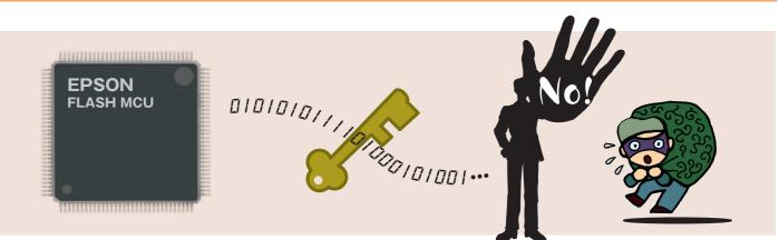
The debug interface disconnection function and the flash memory write/read protections are provided to protect the contents of the built-in flash memory and the RAM. Prohibiting data reading and writing protects the important software assets for our customers.
