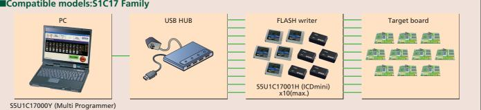
• Up to 10 units of the S5U1C17001H (ICDmini) can be used to construct an environment enabling user data to be downloaded simultaneously to multiple targets. • The S5U1C17000Y, GangWriter software that controls the ICDmini, provides user- friendly screen and simple operation.
