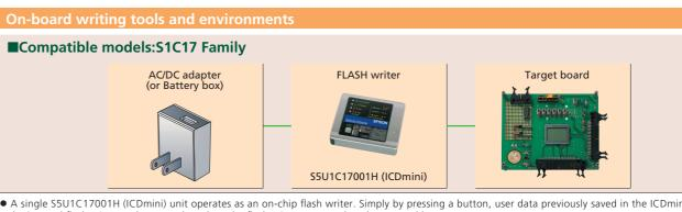
• A single S5U1C17001H (ICDmini) unit operates as an on-chip flash writer. Simply by pressing a button, user data previously saved in the ICDmini can be written to the internal flash ROM on the target board, or the flash ROM connected to the external bus.
