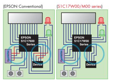
Terminals can be allocated freely using software.
