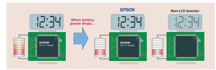
Even when battery power level drops, the contrast level is not affected. The same level of display quality as that of a new machine can be maintained until battery power has been completely consumed. The battery power level is detected by the Supply Voltage Detector (SVD) circuit, so you do not have to be
