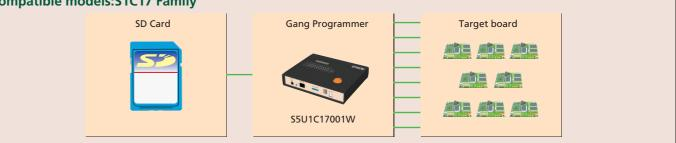
• A single S5U1C1700W unit downloads user data simultaneously to a maximum of 8 targets. An SD card is used to input user data, and the operating status can be checked by LCD, LED and buzzer.
