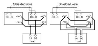
Do not wire the Power Supplies as shown below. It will cause output voltage imbalance, so that one of the units will supply exceeding current, causing the overload protection to engage, resulting in an unstable current and reducing product life expectancy.
