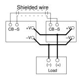
In master/slave operation, the Power Supply with the lower voltage adjustment set value (controlled by V. ADJ) is the master unit, and the Power Supply with the higher voltage adjustment set value is the slave unit.
