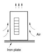
It is recommended to install the Power Supply on a metal plate, and to use forced air cooling. When installing two or more Power Supplies side-by-side, allow at least 20 mm spacing between them, as shown in the diagram below.
