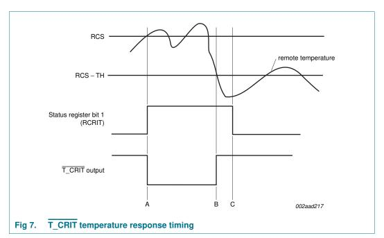
Event A: T CRIT goes LOW and Status bit 1 (RCRIT) is set HIGH when Remote Temperature exceeds RCS, Remote T CRIT Setpoint.
