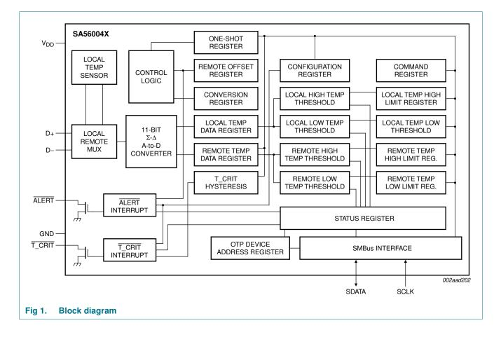
Digital temperature sensor with overtemperature alarms
