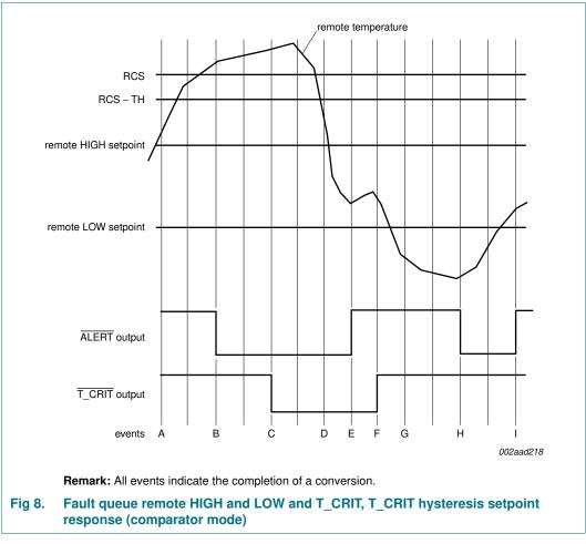
Event A: The remote temperature has exceeded the Remote HIGH setpoint.
