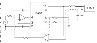
gain of less than one translates the differential output voltage to a single feedback voltage. Dashed line connections and a higher gain difference amplifier would be used for current control. The error amplifier integrates the difference between the input and feedback voltages to close the loop.
