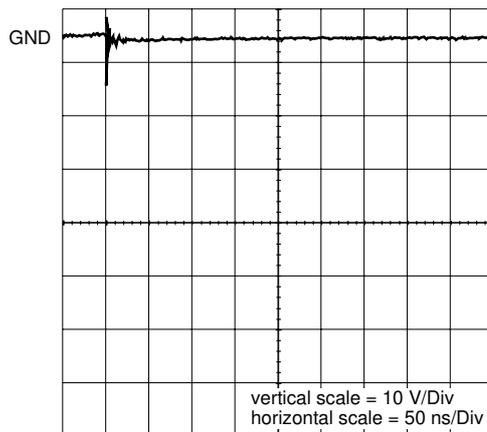
clamped -1 kV ESD voltage waveform (IEC 1000-4-2 network)
