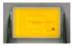
(3) When populating boards in SMT production, there are basically no restrictions regarding the form of the pick and place nozzle, except that mechanical pressure on the surface of the resin must be prevented.
