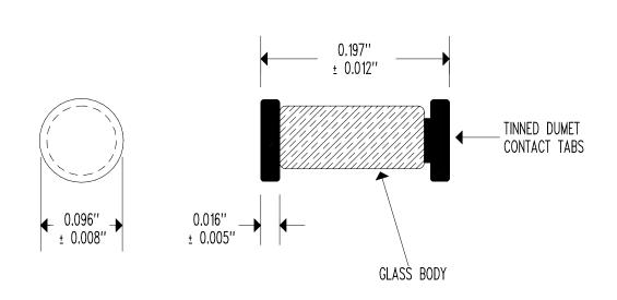
RESISTANCE @  $+25^{\circ}\text{C} = 3,000 \ \Omega \pm 10\%$ RESISTANCE/TEMPERATURE CURVE = "J" BETA " $\beta$ " (0 TO  $+50^{\circ}\text{C}$ ) = 3,892 K NOMINAL TEMPERATURE COEFFICIENT @  $+25^{\circ}\text{C} = -4.4\%$  C NOMINAL DISSIPATION CONSTANT = 3 mW/°C NOMINAL THERMAL TIME CONSTANT = 8 SECONDS MAXIMUM MAXIMUM TEMPERATURE RATING =  $+220^{\circ}\text{C}$
