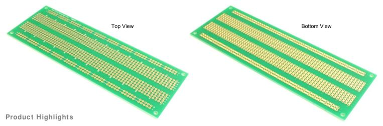
Immersion Gold Finish All holes are gold plated and are on a 0.1" grid 1/16" (1.6mm) thick FR-4 UL94V-0 Accepts a variety of wire sizes (20-32 AWG) 4 mounting holes
