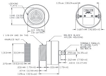
NOTE A: TERMINALS-032 BRASS TIN PLATED, TAPPED FOR #6-32 SCREW. TWO #6-32 NICKEL PLATED BRASS SCREWS INCLUBED. WILL ACCEPT 1/4\* QUICK CONNECT. NOTE B: MOUNTING- REMOVE BLACK PLASTIC NUT AND INSERT THREADED FRONT THROUGH 1.25' HOLE PUNCHED IN PANEL, IF ORIENTATION IS NEEDED, NOTE LOCKING FLATS ON DRAVING. SCREW NUT BACK ON. DO NOT OVERTIGHTEN.
