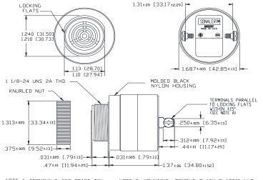
NOTE A: TERMINALS-.032 BRASS TIN PLATED, TAPPED FOR #6-32 SCREW. TWO #6-32 NICKEL PLATED BRASS SCREWS INCLUBED. WILL ACCEPT 1/4' QUICK CONNECT. NOTE B: MOUNTING- REMOVE BLACK PLASTIC NUT AND INSERT THREADED FRINT THROUGH 1.25' HOLE PUNCHED IN PANEL, IF DRIENTATION IS NEEDED, NOTE LOCKING FLATS ON DRAVING. SCREW NUT BACK ON. DO NOT OVERTIGHTEN.
