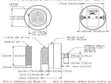
NOTE A: TERMINALS-032 BRASS TIN PLATED, TAPPED FOR #6-32 SCREW. TWO #6-32 NICKEL PLATED BRASS SCREWS INCLUDED. WILL ACCEPT 1/4\* OUICK CONNECT.
