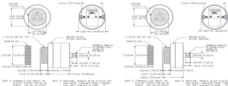
NOTE A: TERMINALS-032 BRASS TIN PLATED, TAPPED FOR #6-32 SCREW. TWO #6-32 NICKEL PLATED BRASS SCREWS INCLUBED. WILL ACCEPT 1/4\* QUICK CONNECT.
