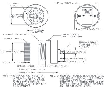
NOTE B: MOUNTING- REMOVE BLACK PLASTIC NUT AND INSERT THREADED FRONT THROUGH 1.25' HOLE PUNCHED IN PANEL, IF DRIENTATION IS NEEDED, NOTE LOCKING FLATS ON DRAWING. SCREW NUT BACK ON. DO NOT OVERTIGHTEN.
