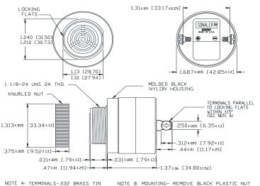
NOTE A: TERMINALS-.032 BRASS TIN PLATED, TAPPED FOR #6-32 SCREW. TWD #6-32 NICKEL PLATED BRASS SCREWS INCLUBED. WILL ACCEPT 1/4\* QUICK CONNECT.
