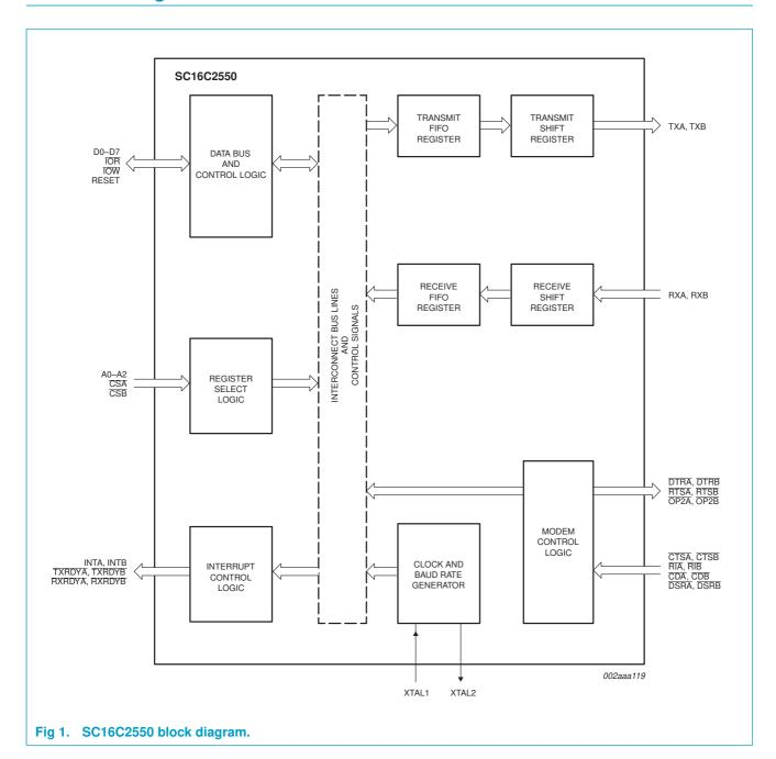
Dual UART with 16 bytes of transmit and receive FIFOs and IrDA encoder/decoder
