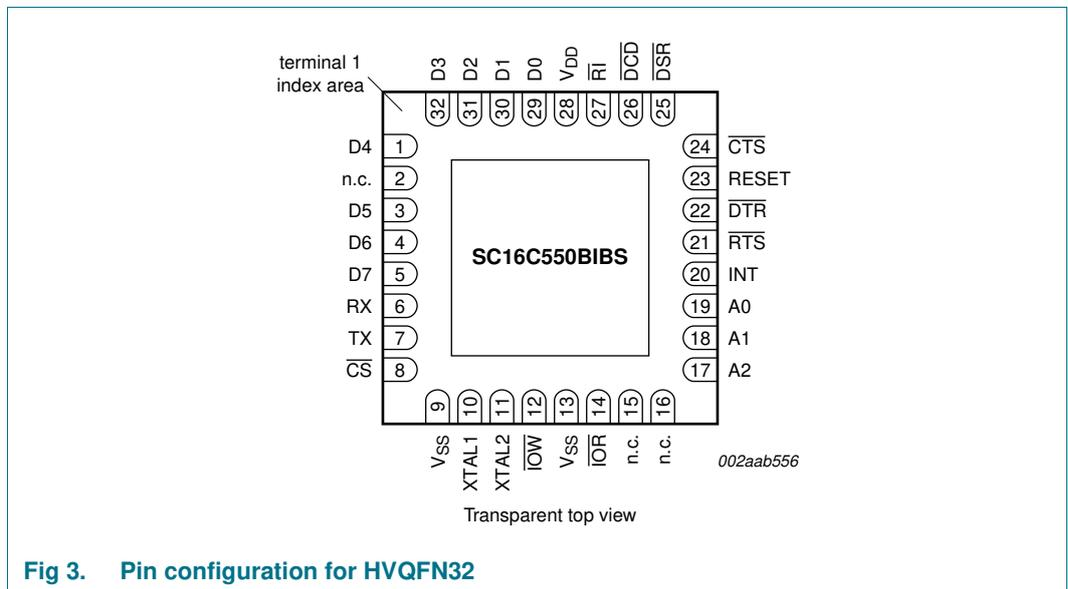
Fig 3. Pin configuration for HVQFN32
