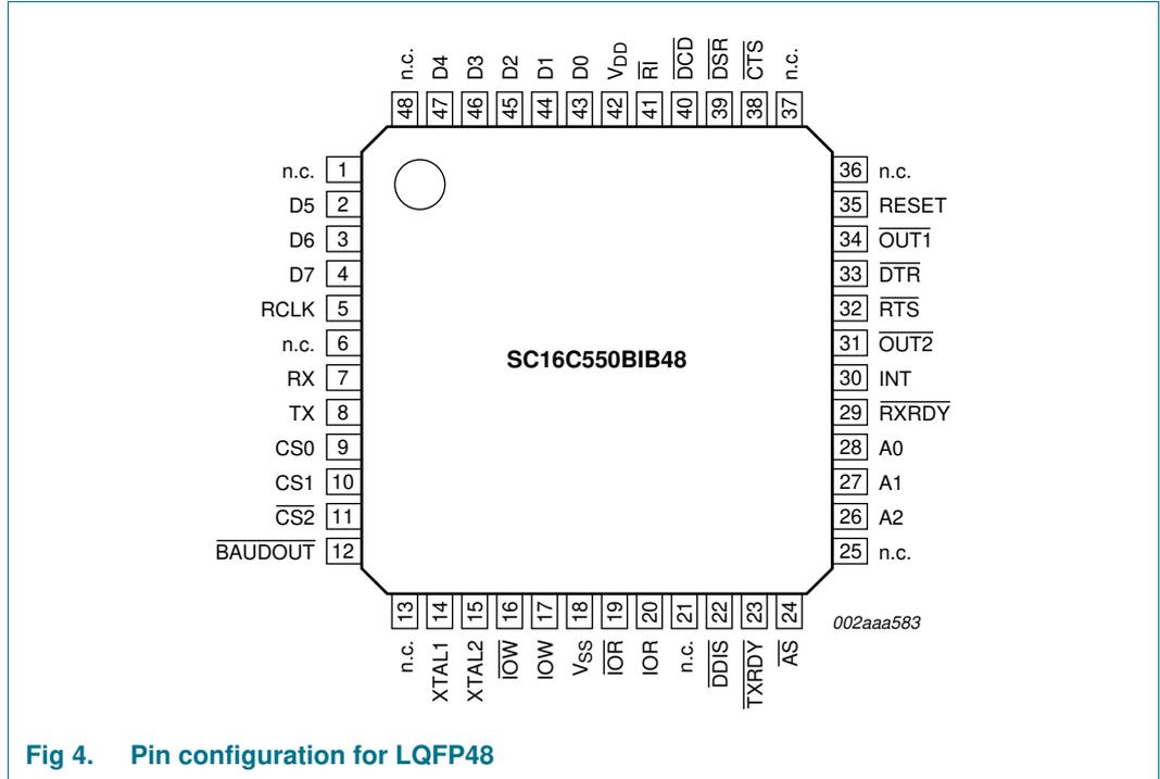
**Fig 4. Pin configuration for LQFP48**
