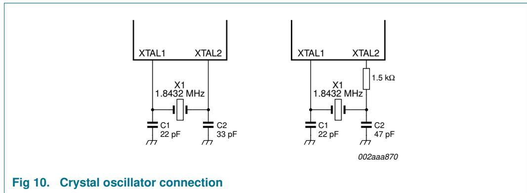
Fig 10. Crystal oscillator connection
