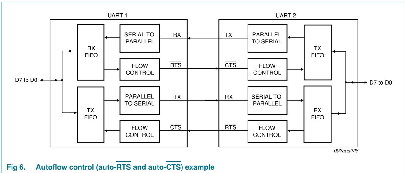
Fig 6. Autoflow control (auto- $\overline{\text{RTS}}$  and auto- $\overline{\text{CTS}}$ ) example
