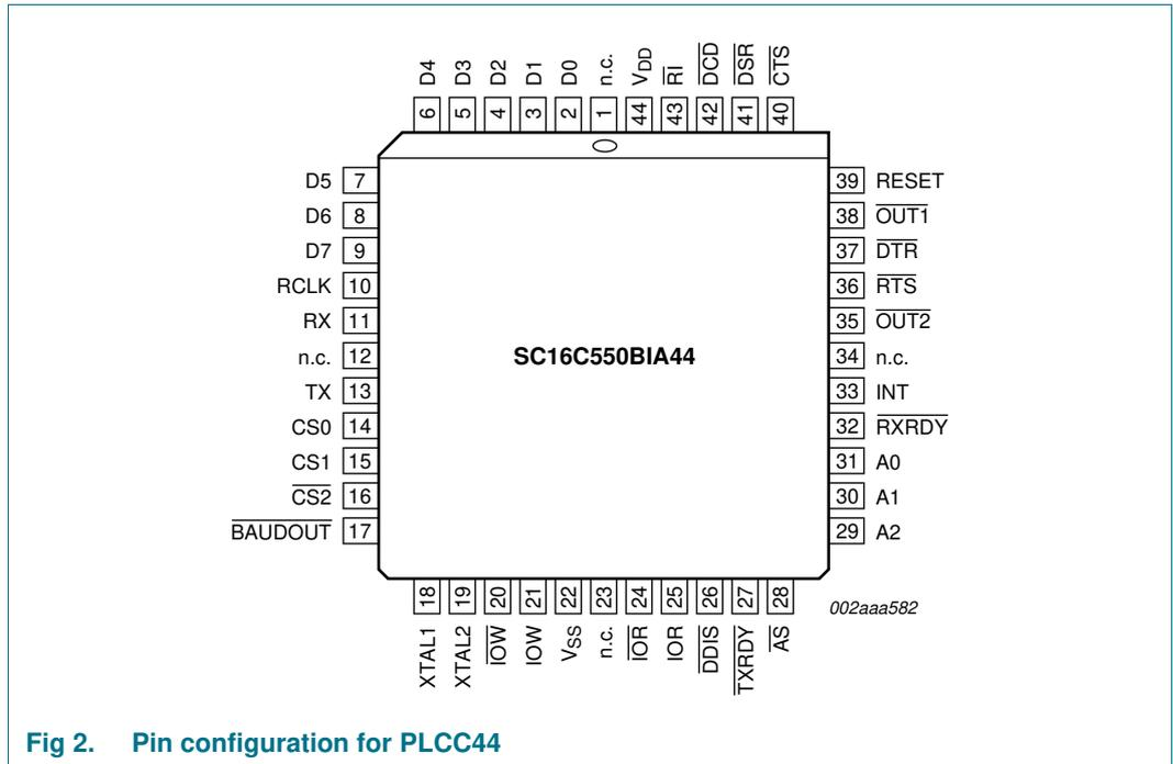
Fig 2. Pin configuration for PLCC44
