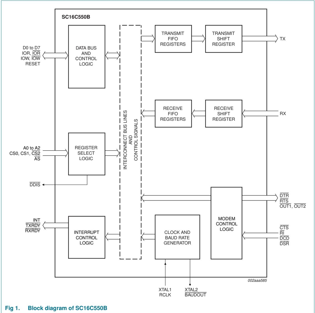
Fig 1. Block diagram of SC16C550B
