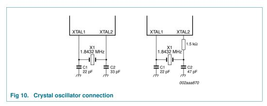
The generator divides the input  $16\times$  clock by any divisor from 1 to  $(2^{16}-1)$ . The <u>SC16C550B</u> divides the basic crystal or external clock by 16. The frequency of the <u>BAUDOUT</u> output pin is exactly  $16\times$  (16 times) the selected baud rate (<u>BAUDOUT</u> =  $16\times$  baud rate). Customized baud rates can be achieved by selecting the proper divisor values for the MSB and LSB sections of the baud rate generator.
