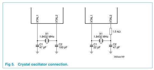
The generator divides the input  $16 \times$  clock by any divisor from 1 to  $2^{16} - 1$ . The SC16C650A divides the basic crystal or external clock by 16. The frequency of the  $\overline{BAUDOUT}$  output pin is exactly  $16 \times (16 \text{ times})$  of the selected baud rate (BAUDOUT = 16 Baud Rate). Customized baud rates can be achieved by selecting the proper divisor values for the MSB and LSB sections of baud rate generator.
