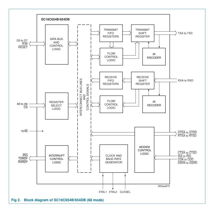
5 V, 3.3 V and 2.5 V quad UART, 5 Mbit/s (max.) with 64-byte FIFOs
