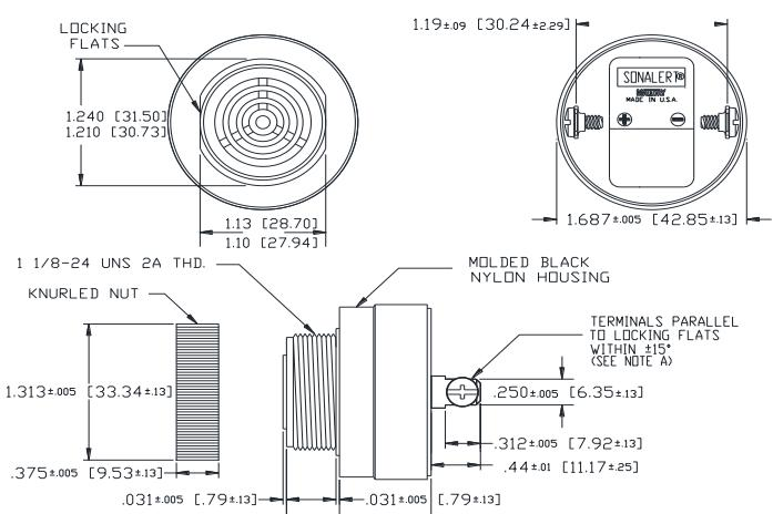
NOTE A: TERMINALS S-.032 BRASS TIN PLATED, TAPPED FOR #6-32 SCREW, TWO #6-32 NICKEL PLATED BRASS SCREWS INCLUDED, WILL ACCEPT 1/4" QUICK CONNECT.
