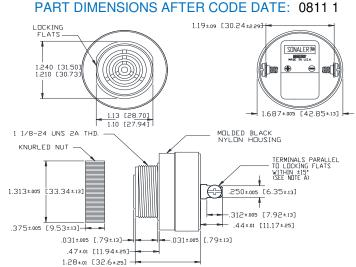
NOTE A: TERMINALS-032 BRASS TIN PLATED, TAPPED FOR #6-32 SCREW. TVO! #6-32 NICKEL PLATED BRASS SCREWS INCLUDED. WILL ACCEPT 1/4' QUICK CONNECT.
