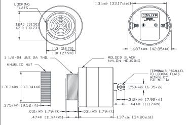
NOTE A: TERMINALS-.032 BRASS TIN PLATED, TAPPED FOR #6-32 SCREW. TWD #6-32 NICKEL PLATED BRASS SCREWS INCLUDED. WILL ACCEPT 1/4\* QUICK CONNECT. NOTE B: MOUNTING- REMOVE BLACK PLASTIC NUT AND INSERT THREADED FRINT THROUGH 1.25' HOLE PUNCHED IN PANEL, IF DRIENTATION IS NEEDED, NOTE LOCKING FLATS ON DRAWING. SCREW NUT BACK ON. DO NOT OVERTIGHTEN.
