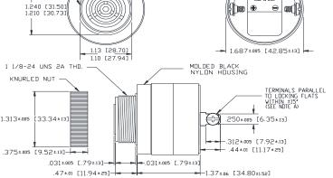
NOTE A: TERMINALS-032 BRASS TIN PLATED, TAPPED FOR #6-32 SCREW. TWO #6-32 NICKEL PLATED BRASS SCREWS INCLUBED. WILL ACCEPT 1/4" QUICK CONNECT. NDTE B: MOUNTING- REMOVE BLACK PLASTIC NUT AND INSERT THREADED FRUNT THRRUGH 1.25' HOLE PUNCHED IN PANEL, IF DRIENTATION IS NEEDED, NOTE LOCKING FLATS ON DRAWING. SCREW NUT BACK ON. DO NOT OVERTIGHTEN.
