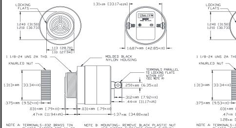
NOTE A: TERMINALS-.032 BRASS TIN PLATED, TAPPED FOR #6-32 SCREW. TWO #6-32 NICKEL PLATED BRASS SCREWS INCLUDED. WILL ACCEPT 1/4' QUICK CONNECT. NOTE B: MOUNTING- REMOVE BLACK PLASTIC NUT AND INSERT THREADED FRONT THROUGH 1.25 HOLE PUNCHED IN PANEL, IF DRIENTATION IS NEEDED, NOTE LOCKING FLATS ON DRAWING. SCREW NUT BACK ON. DO NOT OVERTIGHTEN.
