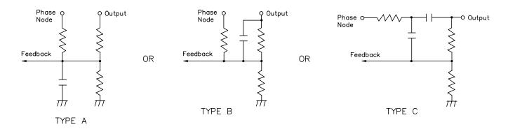
The phase injection improves stability and can provide droop response.
