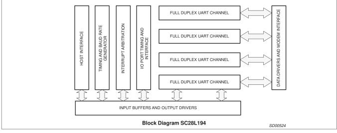
Figure 2. Block Diagram
