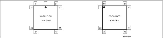
Figure 1. Pin Configurations
