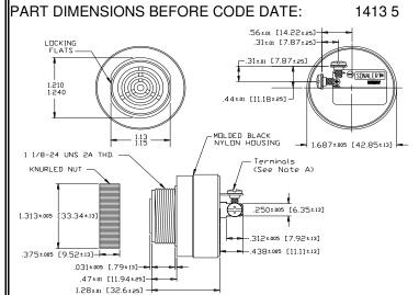
NOTE A: TERMINALS-032 BRASS TIN PLATED, TAPPED FOR #6-32 SCREW. TWD #6-32 NICKEL PLATED BRASS SCREWS INCLUDED. WILL ACCEPT 1/4\* QUICK CONNECT. NOTE B: MOUNTING- REMOVE BLACK PLASTIC NUT AND INSERT THREADED FRONT THROUGH 1.25' HOLE PUNCHED IN PANEL, IF DRIENTATION IS NEEDED, NOTE LOCKING FLATS ON DRAWING, SCREW NUT BACK ON. DO NOT DVERTIGHTEN.
