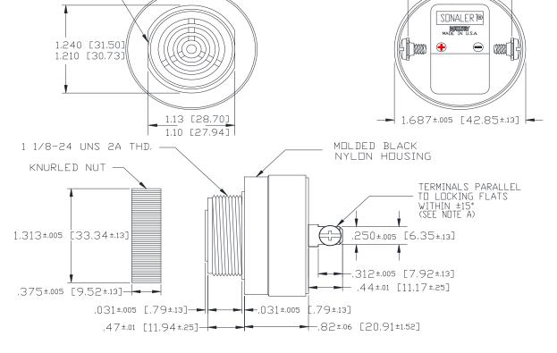
NOTE A: TERMINALS-.032 BRASS TIN PLATED, TAPPED FOR #6-32 TWD #6-32 NICKEL SCREW. PLATED BRASS SCREWS INCLUDED. WILL ACCEPT 1/4" QUICK CONNECT.
