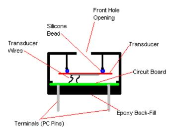
The above cross section picture shows the basic elements used in a piezoelectric audible alarm. The area in front of the transducer element including the front hole opening forms an acoustic cavity that lets the sound radiate out with the most efficiency (i.e. loudest sound level). If the alarm is an indicator that contains a circuit board, the circuit board is attached to the piezoelectric sounder element via soldered wires.
