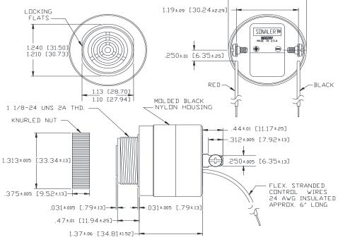
The red and black leads control the several functions. A logic 'Low' is a voltage less than 1/3 of supply voltage. A logic 'High' is a voltage greater than 1/2 supply voltage. A red or black input lead left unconnected is considered an open state.
