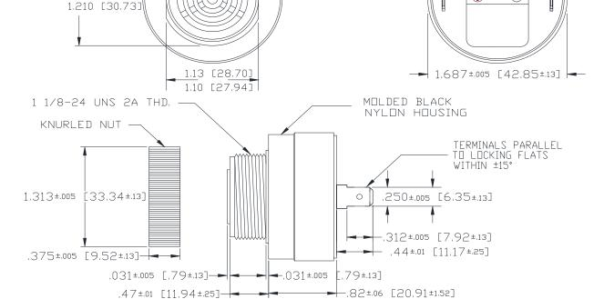
MOUNTING: REMOVE BLACK PLASTIC NUT AND INSERT THREADED FRONT THROUGH 1.25"
