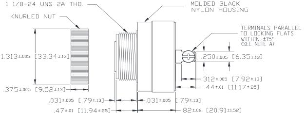
NOTE A: TERMINALS-.032 BRASS TIN PLATED, TAPPED FOR #6-32 SCREW. TWO #6-32 NICKEL PLATED BRASS SCREWS INCLUDED. WILL ACCEPT 1/4" QUICK CONNECT.
