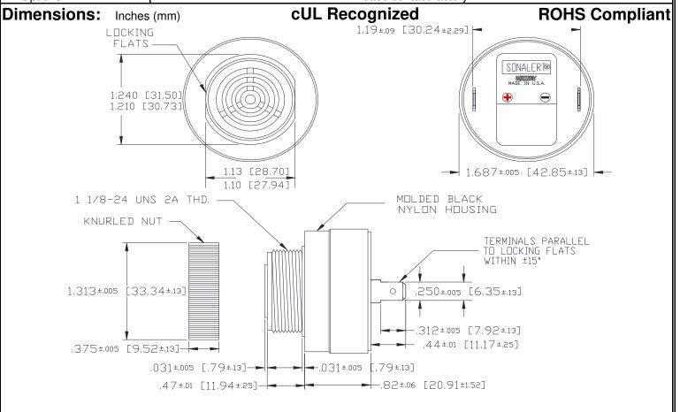
MOUNTING: REMOVE BLACK PLASTIC NUT AND INSERT THREADED FRONT THROUGH 1.25"
