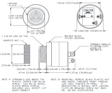
NOTE A: TERMINALS-032 BRASS TIN PLATED, TAPPED FOR #6-32 SCREW. TWO #6-32 NICKEL PLATED BRASS SCREWS INCLUBED. WILA GCEPT 1/4\* QUICK CONNECT.
