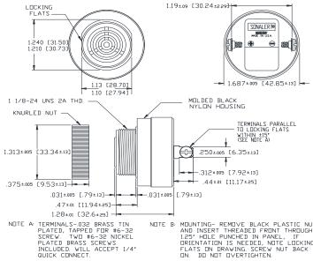
NOTE B: MOUNTING- REMOVE BLACK PLASTIC NUT AND INSERT THREADED FRONT THROUGH 1.25' HOLE PUNCHED IN PANEL, IF DRIENTATION IS NEEDED, NOTE LOCKING FLATS ON DRAWING. SCREW NUT BACK ON. DO NOT OVERTIGHTEN.
