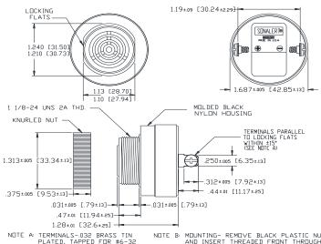
NOTE A: TERMINALS-032 BRASS TIN PLATED, TAPPED FOR #6-32 SCREW. TWO #6-32 NICKEL PLATED BRASS SCREWS INCLUDED. WILL ACCEPT 1/4\* OUICK CONNECT.
