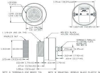
NOTE A: TERMINALS-032 BRASS TIN PLATED, TAPPED FOR #6-32 SCREW. TVD #6-32 NICKEL PLATED BRASS SCREWS INCLUDED WILL ACCEPT 1/4\* OUICK COINNECT. NOTE B: MOUNTING- REMOVE BLACK PLASTIC NUT AND INSERT THREADED FRONT THROUGH 1.25' HOLE PUNCHED IN PANEL, IF DRIENTATION IS NEEDED, NOTE LOCKING FLATS ON DRAWING. SCREW NUT BACK ON. DO NOT OVERTIGHTEN.
