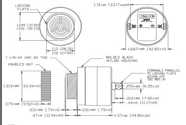
NOTE A: TERMINALS-.032 BRASS TIN PLATED, TAPPED FOR #6-32 SCREW. TWD #6-32 NICKEL PLATED BRASS SCREWS INCLUDED. WILL ACCEPT 1/4\* QUICK CONNECT. NOTE B: MOUNTING- REMOVE BLACK PLASTIC NUT AND INSERT THREADED FRONT THROUGH 1.25' HOLE PUNCHED IN PANEL, IF DRIENTATION IS NEEDED, NOTE LOCKING FLATS ON DRAWING. SCREW NUT BACK UN. DO NOT OVERTIGHTEN.
