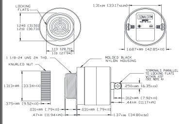
NOTE A: TERMINALS-.032 BRASS TIN PLATED, TAPPED FOR #6-32 SCREW. TWO #6-32 NICKEL PLATED BRASS SCREWS INCLUDED. WILL ACCEPT 1/4" OUICK CONNECT. NOTE B: MOUNTING- REMOVE BLACK PLASTIC NUT AND INSERT THREADED FRONT THROUGH 1.25' HOLE PUNCHED IN PANEL, IF DRIENTATION IS NEEDED, NOTE LOCKING FLATS ON DRAWING, SCREW NUT BACK ON. DO NOT OVERTIGHTEN.
