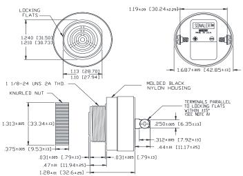
NOTE A: TERMINALS-0.32 BRASS TIN PLATED, TAPPED FOR #6-32 SCREW. TWO #6-32 NICKEL PLATED BRASS SCREWS INCLUBED. WILL ACCEPT 1/4" OUICK CONNECT. NOTE B: MOUNTING- REMOVE BLACK PLASTIC NUT AND INSERT THREADED FRONT THROUGH 1.25' HOLE PUNCHED IN PANEL, IF DRIENTATION IS NEEDED, NOTE LOCKING FLATS ON DRAWING, SCREW NUT BACK ON. DO NOT OVERTIGHTEN.
