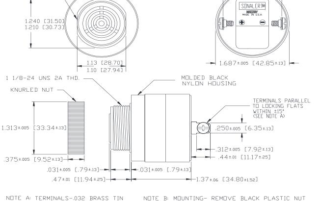
PLATED, TAPPED FOR #6-32 SCREW. TWO #6-32 NICKEL PLATED BRASS SCREWS INCLUDED WILL ACCEPT 1/4"
