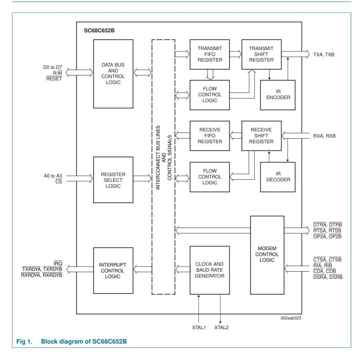
Dual UART with 32-byte FIFOs and IrDA encoder/decoder
