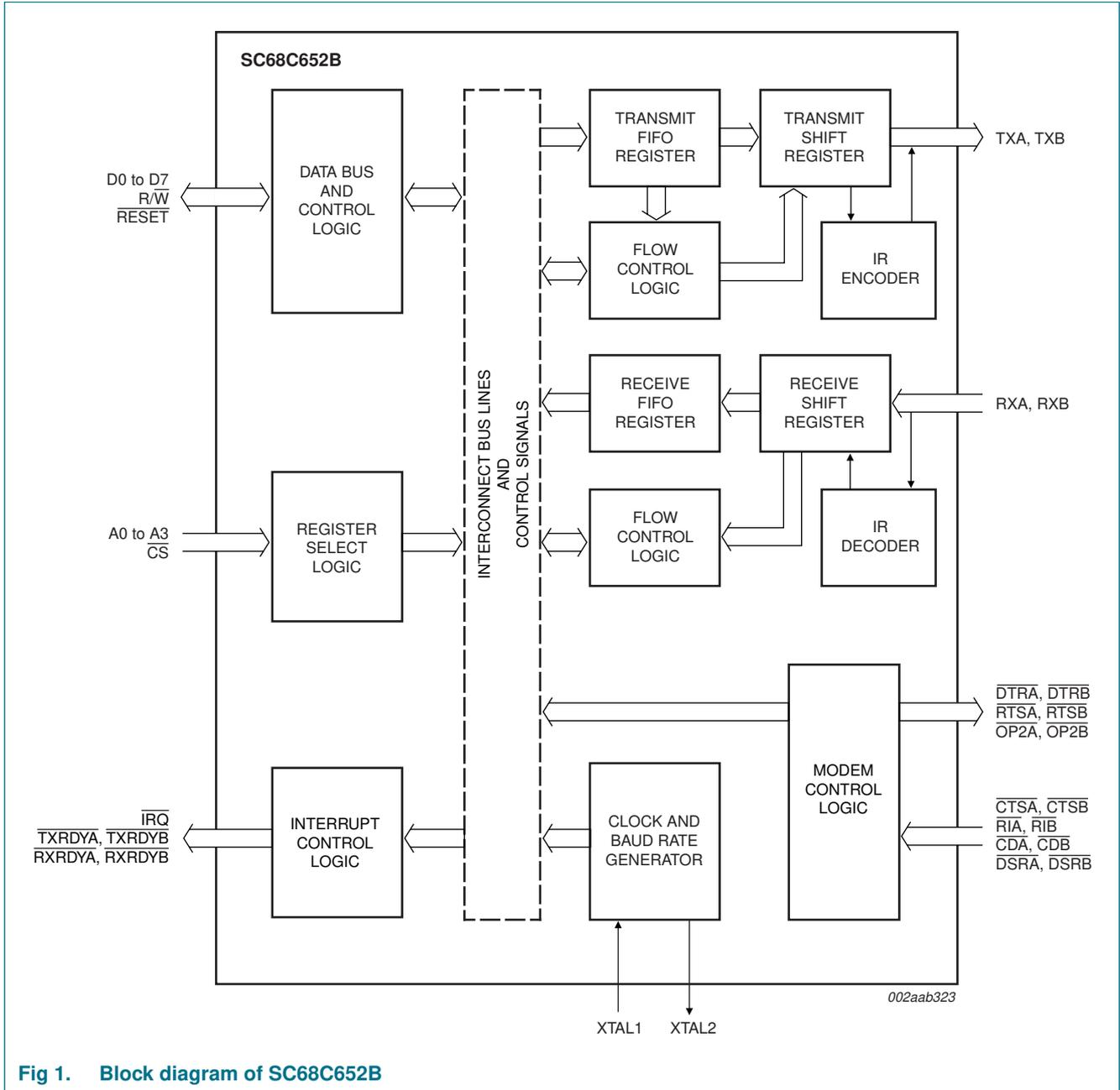
Fig 1. Block diagram of SC68C652B
