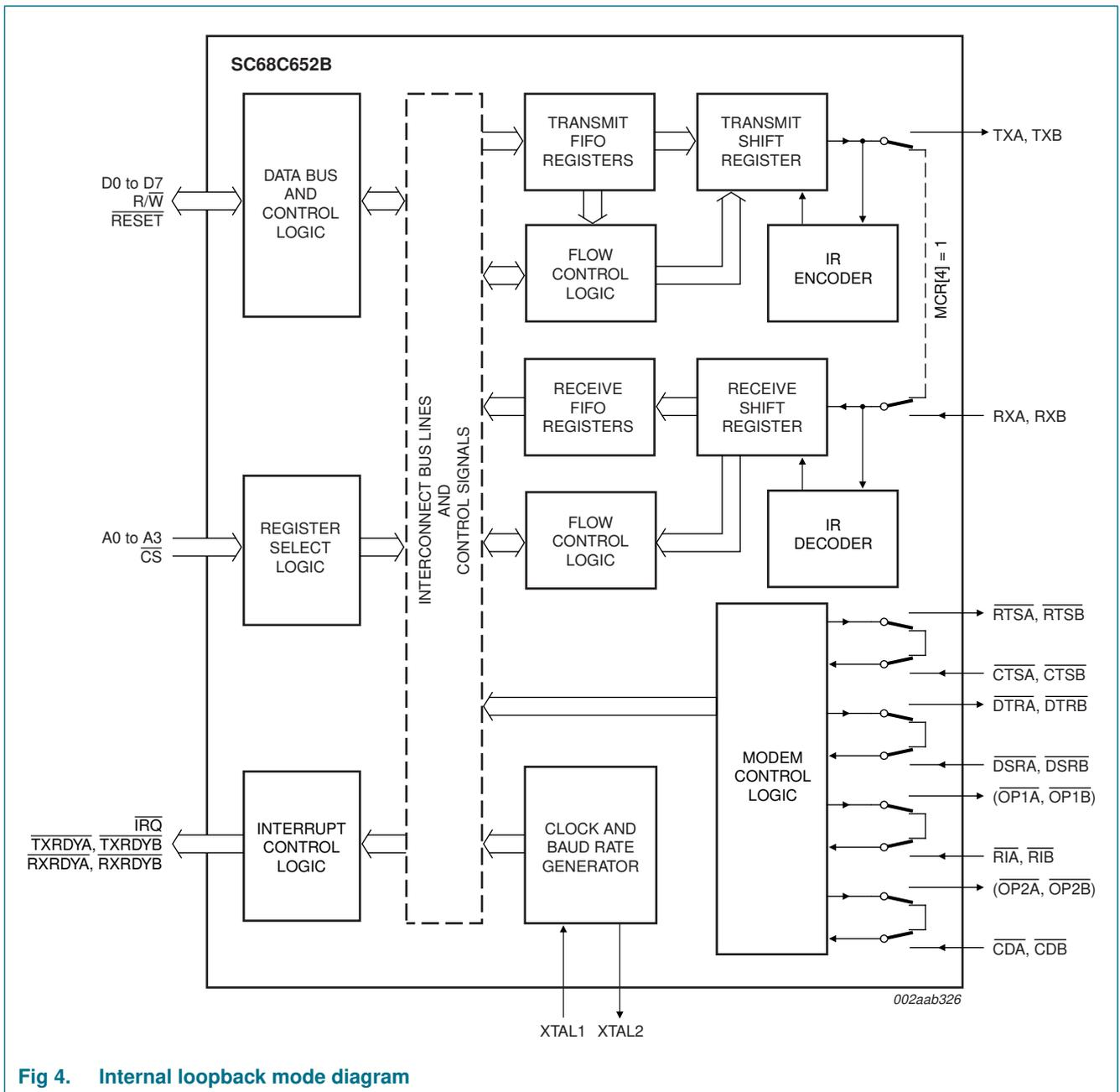
Fig 4. Internal loopback mode diagram
