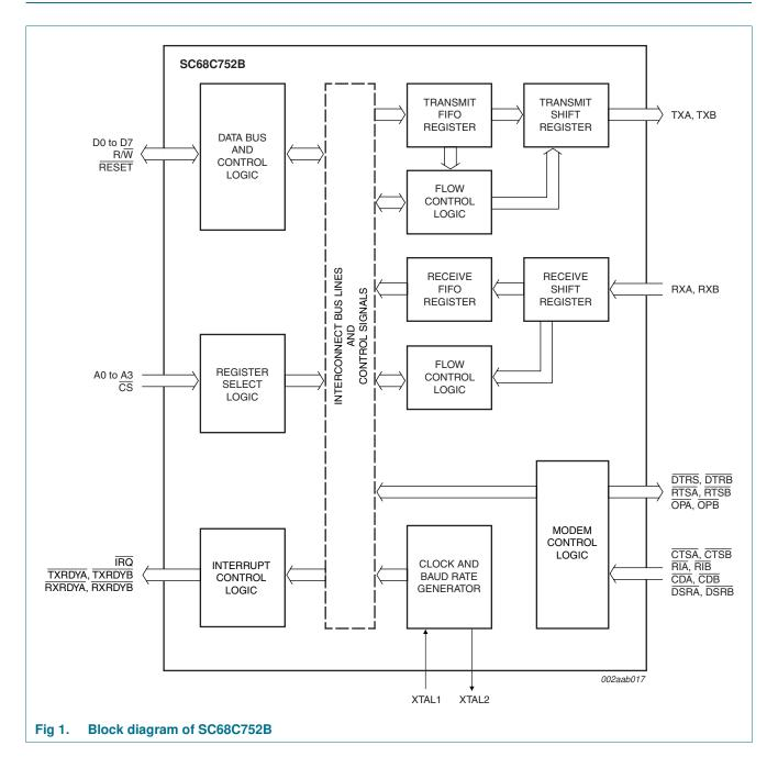
5 V, 3.3 V and 2.5 V dual UART, 5 Mbit/s (max.), with 64-byte FIFOs
