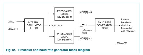
DLL and DLM must be written to in order to program the baud rate. DLL and DLM are the least significant and most significant byte of the baud rate divisor. If DLL and DLM are both zero, the UART is effectively disabled, as no baud clock will be generated.
