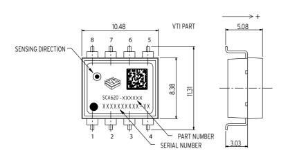
Acceleration in the direction of the arrow will increase the output voltage.
